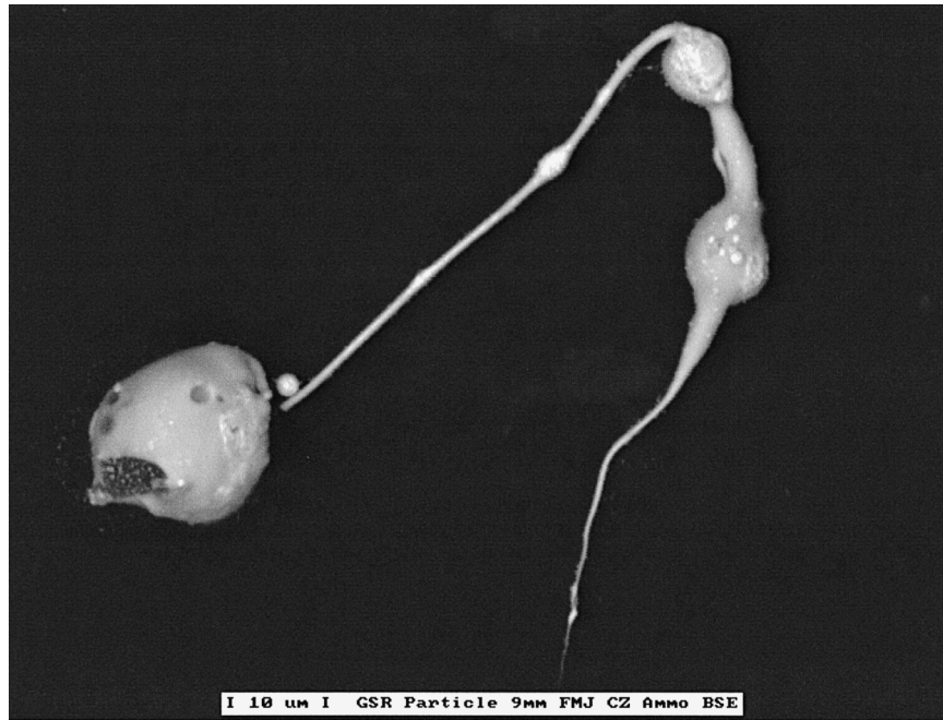
FIG. 5d—Very unusual shape GSR particle. Some ammunition shows abundance of semi-spheroids connected with thin, mostly barium channel.
